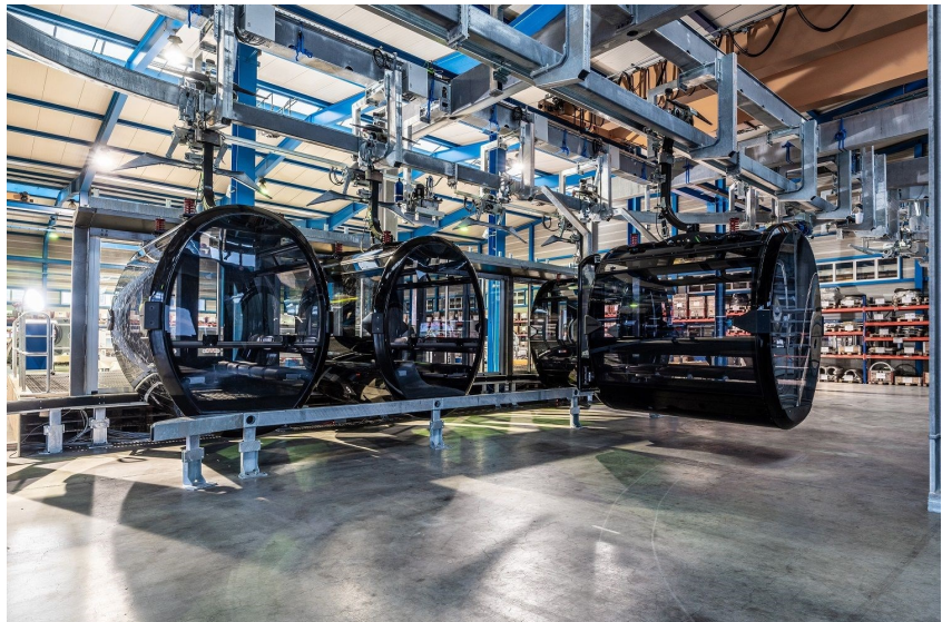
Production of the new gondolas for the urban ropeway in Varanasi, India.
